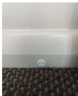
Installed Probes in the skirting
